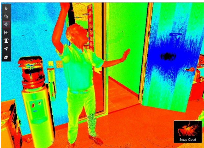
Figure 13a and 13b: Effect of the moving object filter in Cyclone REGISTER 360.
