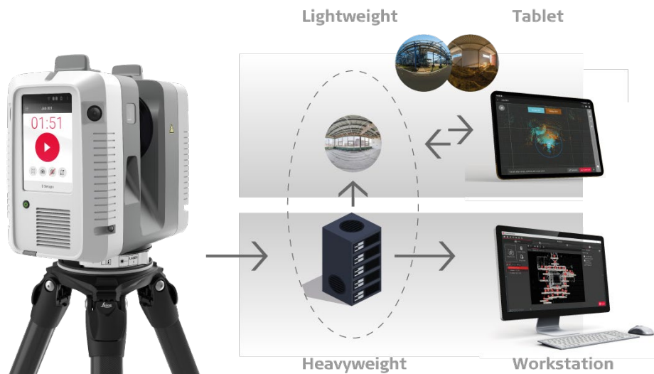
Figure 9: Data transmission and synchronisation between the three components of the RTC360 solution.
